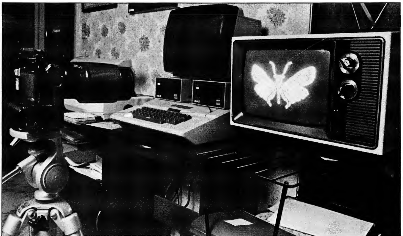
The camera is ready to photograph the drawing on the video screen.
